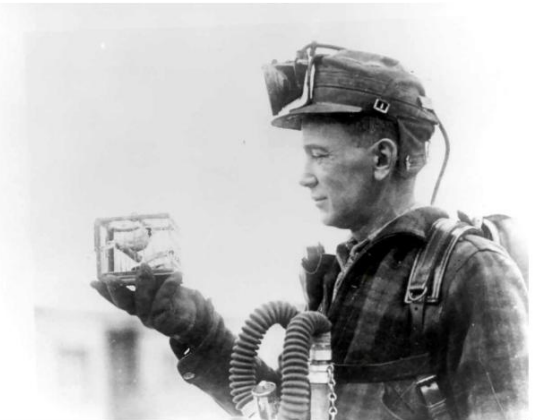
Mining foreman R. Thornburg shows a small cage with a canary used for testing carbon monoxide gas in 1928. (George McCaa, U.S. Bureau of Mines)
