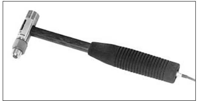
Figure 4. PCB Modally Tuned Impulse Hammer of type responsible for IR-100 award.
