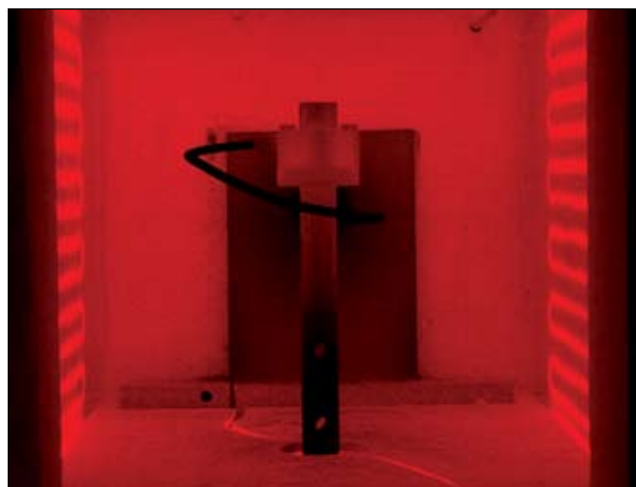
Figure 7. PCB Accelerometer Operating at 1200° F.
